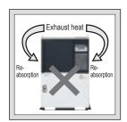
If there are no obstacles within 150 cm of the front and sides of the unit, then the space from the top of the unit to the obstacle above can be as low as 100 cm or higher
