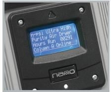
PLC controller with clear text display
